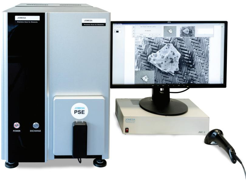
This Jomesa PSE SEM analysis system determines the type of alloys that contaminate a sample. (Photo credits: Jomesa North America)
